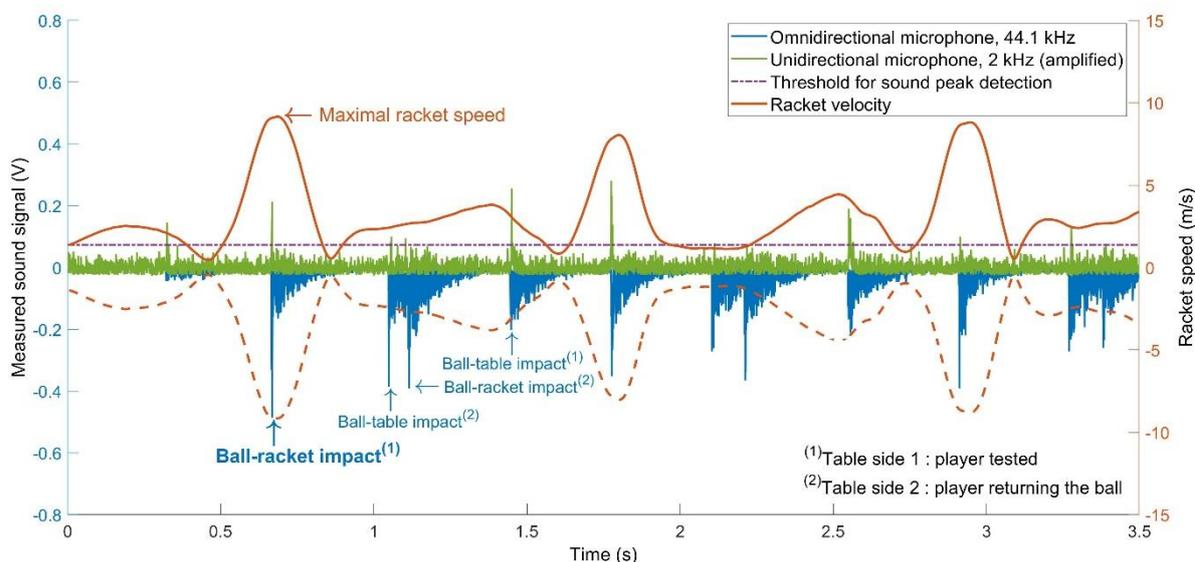
**Figure 1:** Upper envelopes of the measured sound signal of both microphones (2 kHz and 44.1 kHz) and racket speed over the duration of one typical acquisition of three strokes. Each local speed maximum bell represents one stroke. The signal of the 44.1 kHz microphone is plotted symmetrically to the time axis for reading purpose.
