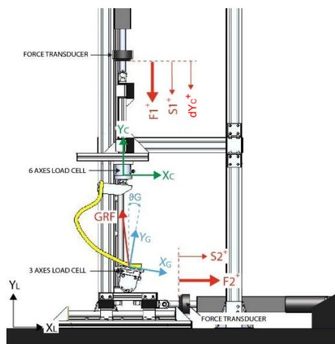
**Figure 1:** In vitro reference systems and main quantities for the test bench [5]
