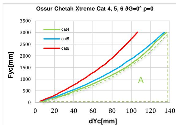
Figure 4: Stiffness curve for Ossur cat 4,5,6 at  $\vartheta_G=0^\circ$  and for  $\rho=0$
