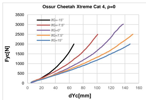
Figure 3: Stiffness curve for Ossur Cat 4 at different  $\vartheta_G$
