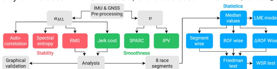
**Figure 1** Flowchart of the trunk movement study, with the steps for stability and smoothness computation, and statistical analysis indicated in red, green, and blue respectively.
