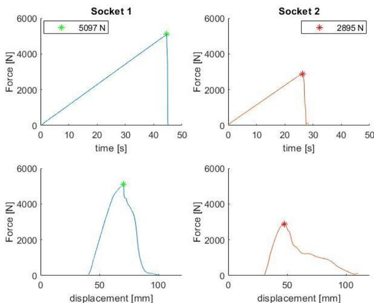
**Figure 4: Loading curves (above) and load-displacement curves (below) for Socket 1 (left) and Socket 2 (right).**
