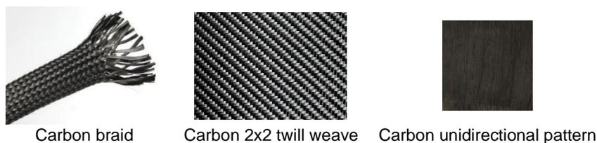
**Figure 3: Possible patterns of carbon fibers used in the layups.**
