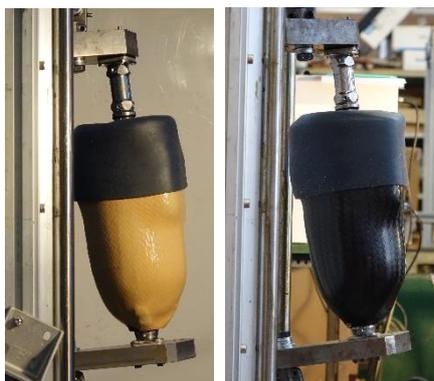
**Figure 2: Sockets tested. Socket 1 (left) and Socket 2 (right).**
