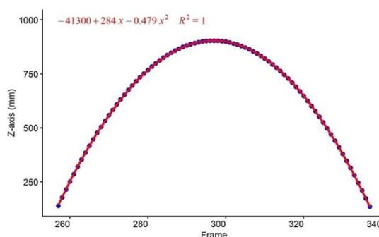
**Figure 3. Example parabola analysis to determine the ball's centre during a bounce trial. The blue trace indicated the ball's true Z-axis position and red line the predicted ball trace, with the  $R^2$  value reporting the variance between the two traces.**
