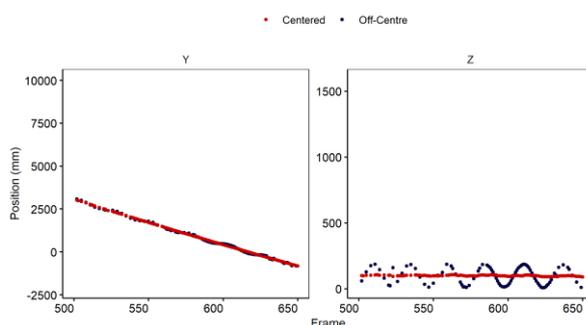
**Figure 2. Example traces of Y (direction of travel) and Z (vertical) position of a ball with the centre skewed to one side (blue line), and the trace with the ball centre correctly identified (red line) whilst rolling along the ground.**
