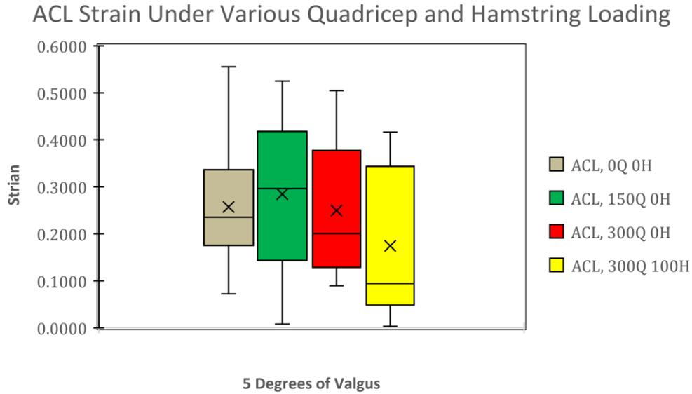
**Figure 2. ACL strain data at 5° of valgus with various muscle preactivation levels (n = 53).**
