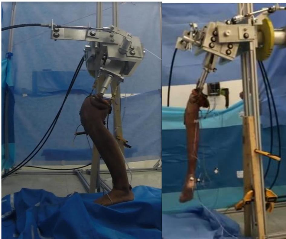
**Figure 1. Two views showing integration of the cadaveric leg into the mechanical hip, forming a hybrid simulator.**
