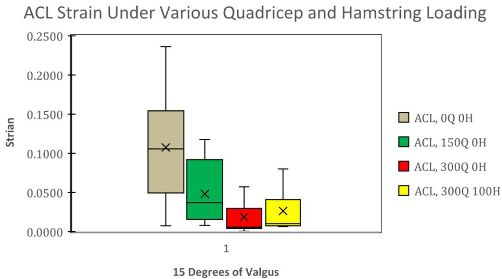
**Figure 3. ACL strain data at 15° of valgus with various muscle preactivation levels (n = 32).**
