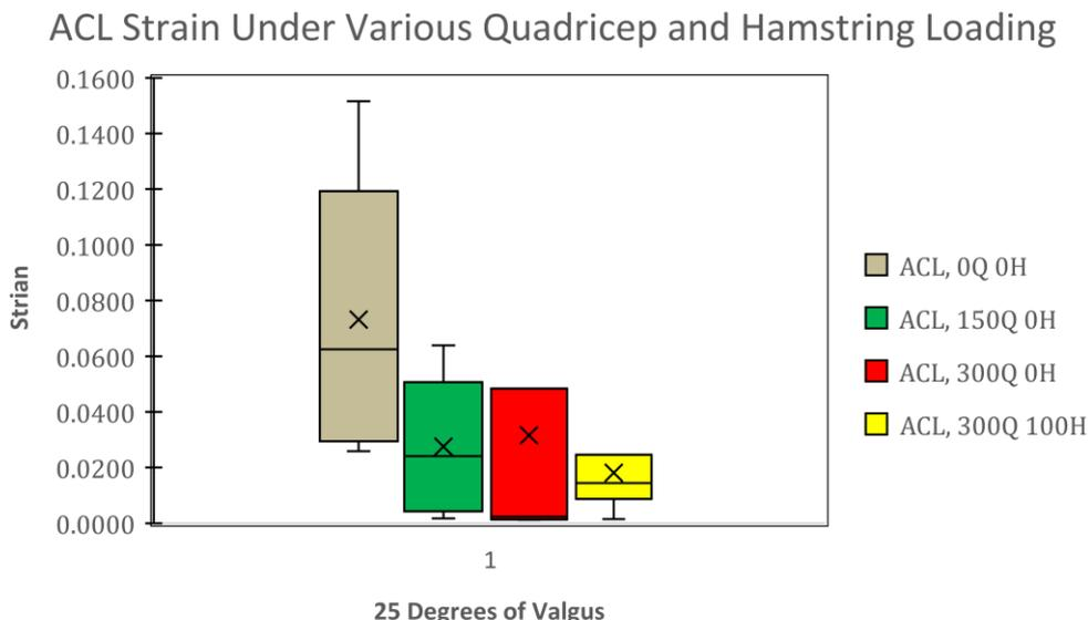
**Figure 4. ACL strain data at 25° of valgus with various muscle preactivation levels (n = 26).**
