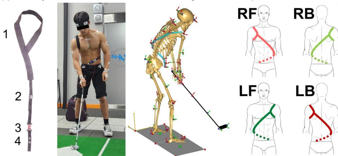
**Figure 1:** Left: Exoband (1. Elastic part, 2. Adjustable buckle, 3. Embedded loadcell, and 4. Lock buttons to attach the exoband to the belt). Middle: golfer while wearing the elastic exoband during RB condition and corresponding musculoskeletal model. Right: Exoband conditions.
