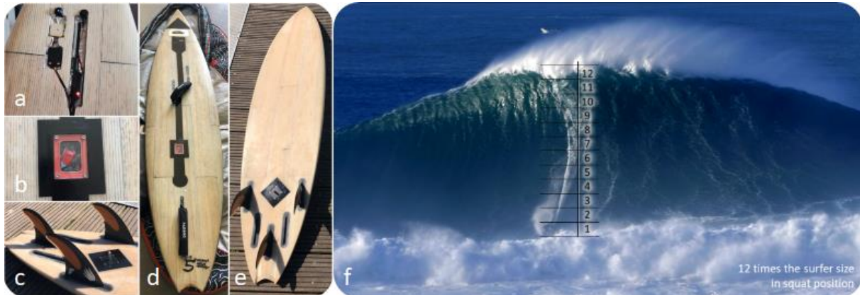
Figure 1 – a) GNSS and Telemetry Radio housed in the surfboard's nose. b) Waterproof central box for accessing electronics, battery, and memory card. c) Fluid Flow Sensor, positioned according to a previous Fluid Dynamics study. d) the top view, and. e) the bottom view of the surfboard. f) The surfed wave, on the critical moment, where the wave is twelve times bigger than the surfer in a squat position.
