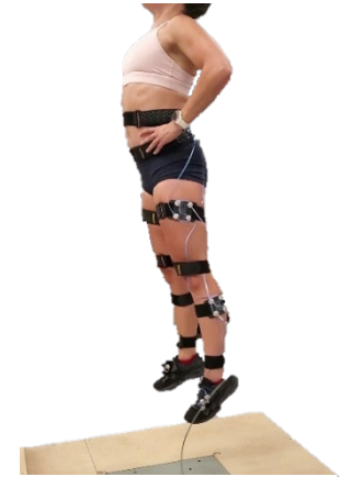
Figure 1 - Participant outfitted with NDI motion capture markers performing counter-movement jump on an OR6-7 force plate.
