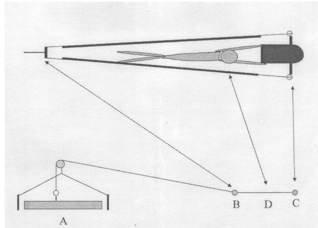
Figure 1. Apparatus connecting swimmer to force platform: (A) shows the force platform and pulley apparatus; (B) depicts the junction between the two cables; (C) illustrates the kickboard with oak dowel attached and (D) shows the cables with the float tubes attached.
